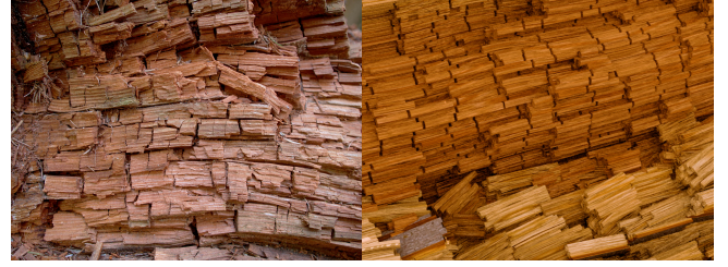
Fig. 4. A picture of a log affected by rot (left) and our simulation results (right). Our method successfully captures the characteristic orthogonal crack propagation and the resulting formation of distinct cubic chunks.
