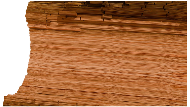
Fig. 8. Lignin-degrading decay yields a smoother, more diffuse weakening pattern than brown rot: material loss spreads gradually through the volume, producing softened, stringy wood with an irregular surface rather than blocky fracturing.
