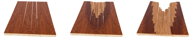
Fig. 15. Initial moisture loss causes anisotropic shrinkage and fiber-aligned cracking in wood (left). The board is subsequently affected by fungal decay, leading to progressive internal deterioration (middle, right).
