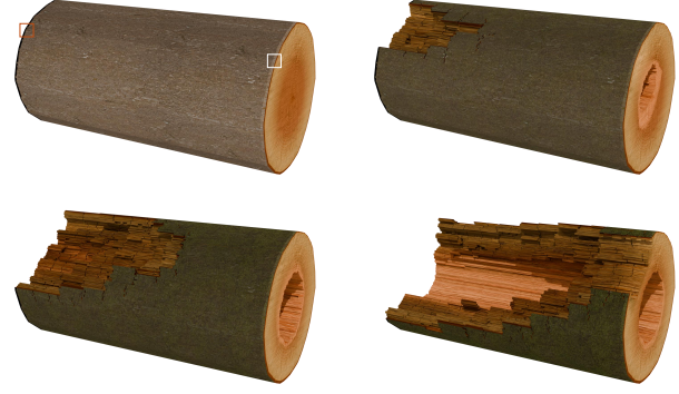
Fig. 13. Brown rot and white rot initiated at opposite ends of the log (rectangular areas). Brown rot preferentially degrades carbohydrate-rich sapwood, producing characteristic cubical fracture patterns, while white rot penetrates into lignin-rich heartwood, hollows the log, and produces a more diffuse degradation pattern.
